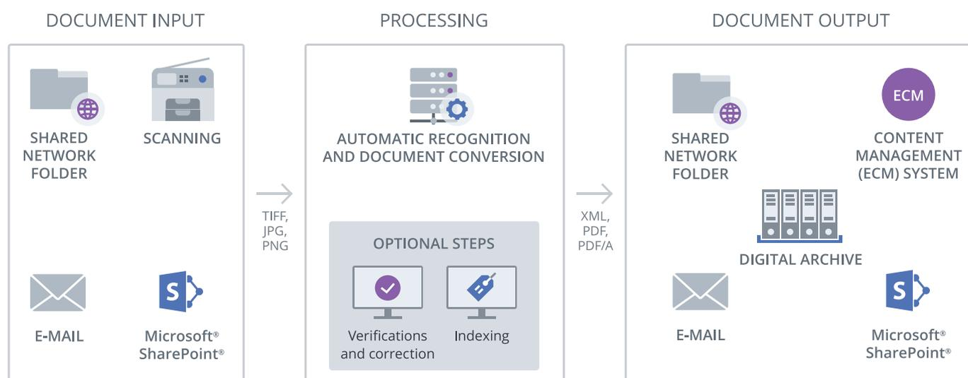
ABBYY FineReader Server receives document images from shared network folders, scanners, e-mails, and Microsoft® SharePoint® and automatically converts them into searchable digital formats using optical character recognition (OCR) technology. If needed, the user can manually correct text information and/or add metadata to the document. The resulting digitized files can be saved to any number of storage areas and/or delivered to other applications.
